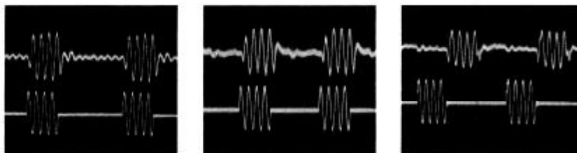
Tone-burst responses at (left to right) 60, 250 and 4000 Hz.
